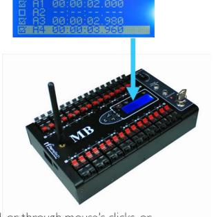
You can assign Firing Time Points in PC through input of keyboard, or through mouse's clicks, or according to the playing of music, can achieve different kinds of purpose.
